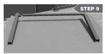
Slide your top rail into the pocket with the nubs facing the ground for both uprights. Ensure the rail is inserted all the way into the upright. Confirm your outside to outside dimensions are 46-7/32".
