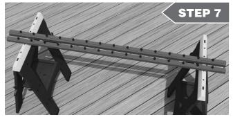
Place your rails on a flat surface, nubs side up, and mark your measurement with equal distances between the nubs, at both ends on both rails.
