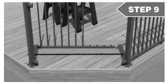
Assemble the rail section by first pressing the balusters onto the bottom rail nubs, then press the top rail nubs into the baluster tops. Use even force to fully seat all of the balusters.
