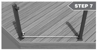
Measure the distance between the inside of the bracket cups while allowing a 1/4" gap to the back of the cups at each end. Take note of the measurement.
