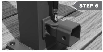
Attach the bottom bracket cup to the backer plate with a #14 Tek screw. And repeat the process for the top bracket.
