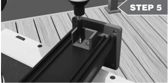
Secure the bottom bracket using the #14 x 1" Tek 18/8 screws provided.
