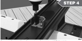
Secure the top bracket using the #14 x 1" Tek 18/8 screws provided.
