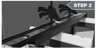
Temporarily fasten the template onto the post using bar clamps.
