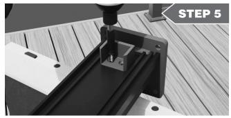
Secure the bottom bracket using the #14 x 1" Tek 18/8 screws provided.
